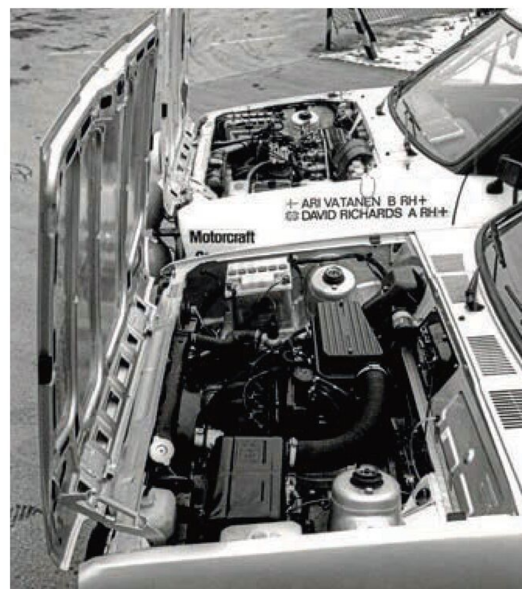
Under the bonnet of the embryonic Fiesta RS was a 1.3-litre twin-carb Kent engine, here shown alongside the Vatanen rally car that used a highly-tuned version of the 1.6-litre engine
